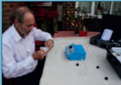
2 Make sure the cuvettes are thoroughly clean and scratch-free before using them.
