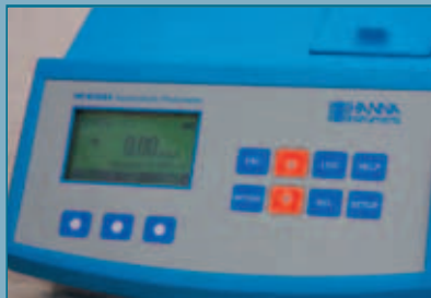
5 Press zero – 'zero testing' will increase the accuracy of testing the actual samples.
