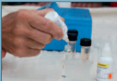
6 Once zero testing is complete, remove the cuvette from the machine and add the reagent.
